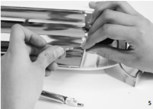
5. IF WORN, APPLY THE SPARE HEAT-ELASTIC CAPS TO REPLACE THOSE WHICH HAVE BEEN REMOVED. STRIP THE CORDS (5-6 mm), APPLY THE NEW SPARE FASTONS AND FASTEN THEM TO THE CORD.
