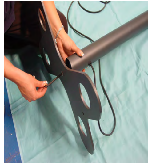
3. Join the two parts of the four-lobe base (D) and fix it to the shorter pole (A) through which the supply cable runs, using the 8x25 socket head screws, tightening them with the allen wrench supplied.
