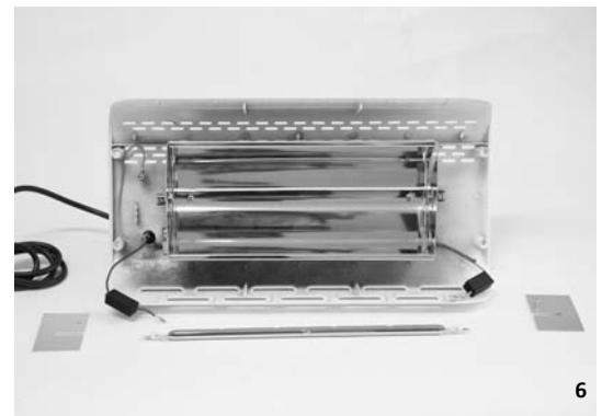
6. APPLY THE SPARE HEAT-ELASTIC CAPS TO REPLACE THOSE WHICH HAVE BEEN REMOVED.
