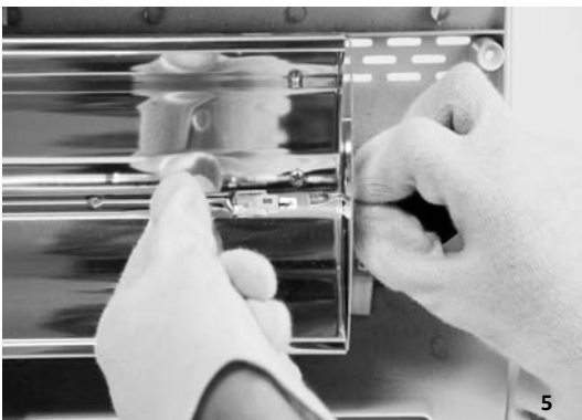
5. INSERT THE NEW BULB INTO THE SPRING CLIPS, THE SHORTENED CORDS OF WHICH ARE TO BE INSERTED INTO THE CLAMPS. REASSEMBLE THE DEVICE BY PERFORMING THE ABOVE TASKS IN REVERSE ORDER.
